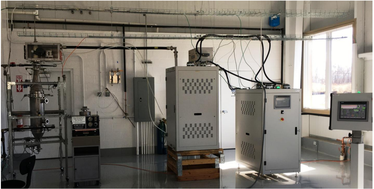
Fig.2. General view of the APT-125 plasma system for nanostructures production. APT facilities in Marshall, VA. June, 2023.
