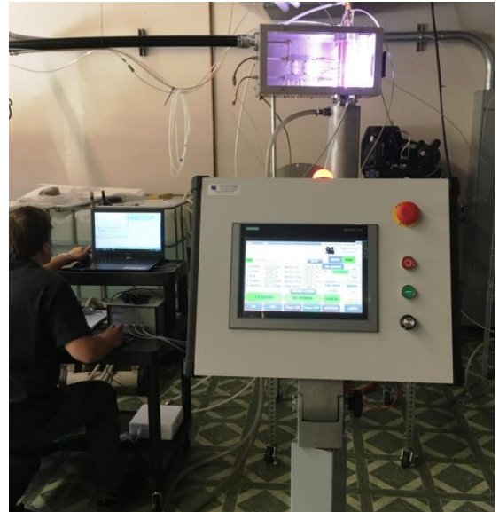
Fig.5. Torch operation and plasma diagnostics by optical spectroscopy
