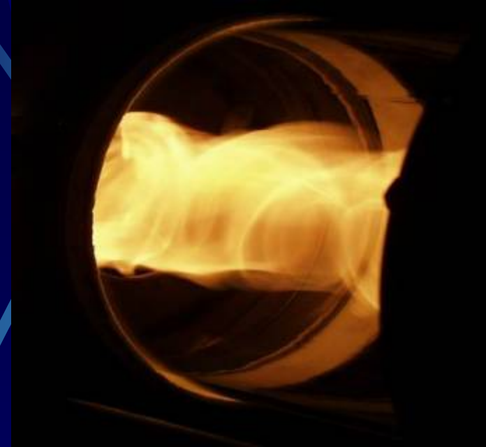
Visualization of the swirling reacting flow
