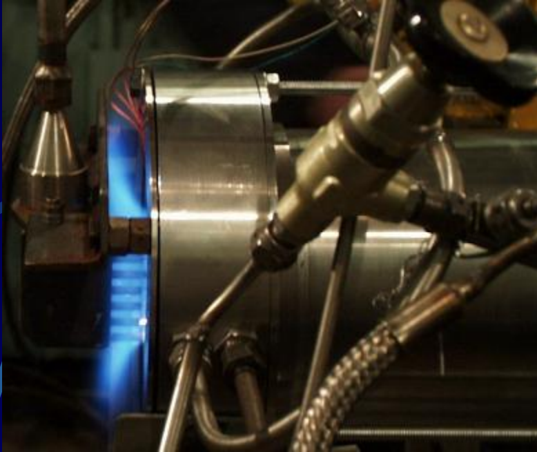
Reverse vortex combustor in operation
