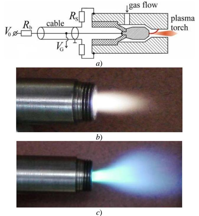
Fig. 1. Experimental arrangement for ignition and flame control in plasmatron (a) and typical photographs of the flame in air (b) and air-propane mixtures (c). Voltage  $V_0$  of negative polarity is applied to the cathode via the ballast resistor  $R_b$  ( $R_S$  is the low-resistive current shunt).
