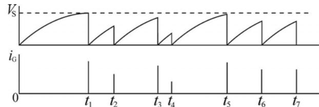
Fig. 2. Voltage at the plasmatron gap  $V_G$  and current through the gap  $i_G$  for the electric circuit shown in Fig. 1 in the conditions when the gap does not completely recover its dielectric strength in a pause between the high-current pulses.
