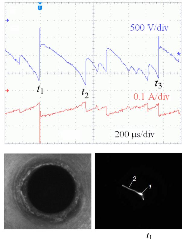
Fig. 4. Voltage and current waveforms for discharge in plasmatron at the stage when discharge is attached to the end of the cathode and CCD photograph of the discharge image.  $R_b = 13.6 \text{ k}\Omega$ ,  $C = 300 \text{ pF}$ ,  $V_0 = 3.0 \text{ kV}$ , gas flow  $G(\text{air}) = 0.5 \text{ g/s}$  ( $v = 20 \text{ m/s}$ ).
