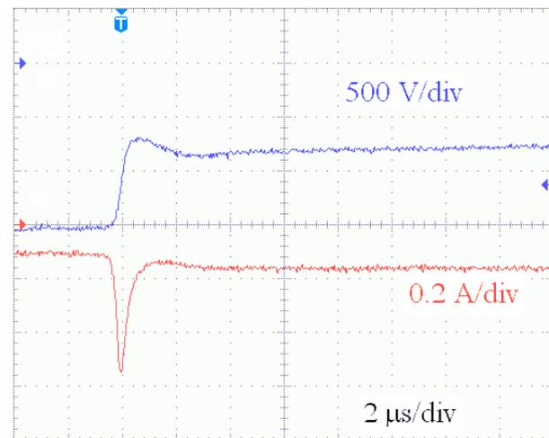
Fig. 5. Typical voltage and current waveforms for non-completed transition from glow to spark in plasmatron.  $R_b = 13.6 \text{ k}\Omega$ ,  $C = 300 \text{ pF}$ ,  $V_0 = 3.0 \text{ kV}$ , gas flow  $G(\text{air}) = 0.1 \text{ g/s}$  ( $v = 4 \text{ m/s}$ ).
