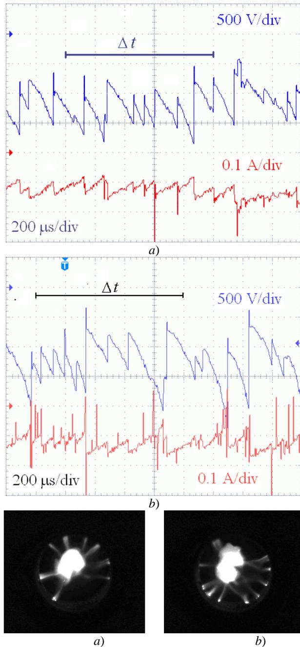
Fig. 7. Voltage and current waveforms for discharge in air-propane mixture and CCD photograph of the discharge image with a large time exposition (exposition time  $\Delta t$  is marked at the waveforms).  $R_b = 13.6$  k $\Omega$ ,  $C = 300$  pF,  $V_0 = 3.0$  kV.  $G(\text{air}) = 1$  g/s ( $v = 20$  m/s,  $G(\text{propane}) \approx 0.01$  g/s.
