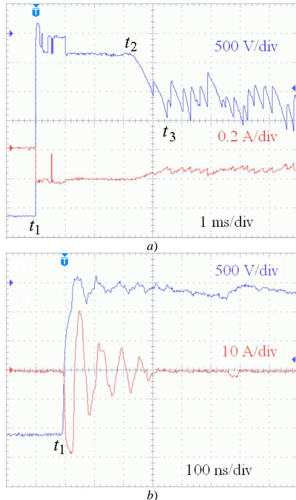
Fig. 3. Voltage and current waveforms for the very first breakdown in the plasmatron. Air flow through the plasmatron  $G(\text{air}) = 0.1$  g/s (gas velocity  $v = 4$  m/s); capacitance of the cable  $C = 300$  pF; ballast resistor  $R_b = 13.6$  k $\Omega$ .
