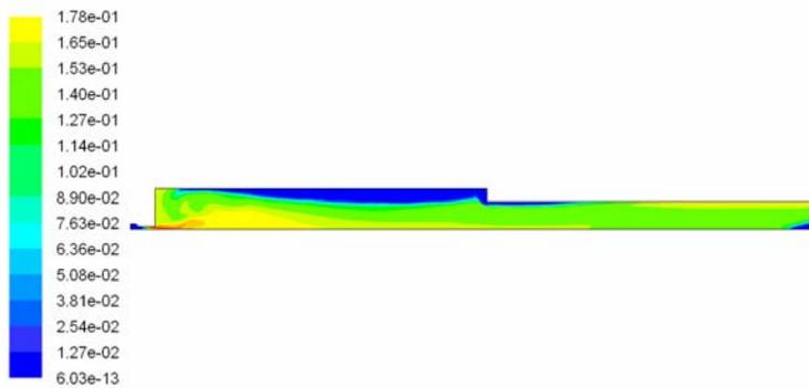
Fig. 2. Contours of  $H_2$  mole fraction
