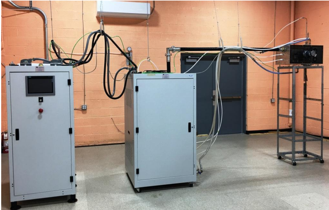
Fig.2. General view of the APT-200 plasma system for material tests
