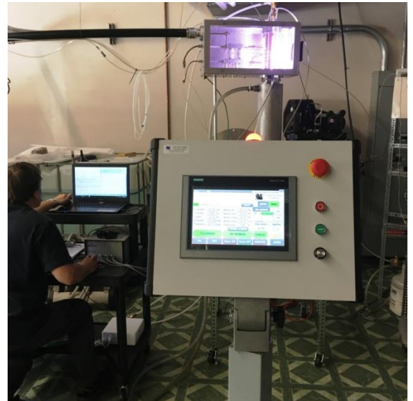
Fig.5. Torch operation and plasma diagnostics by optical spectroscopy
