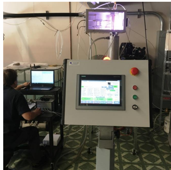
Fig.8. APT-100-5 operation and plasma diagnostics by optical spectroscopy
