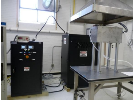
Fig.2. General view of the APT-100-1 plasma system for material tests
