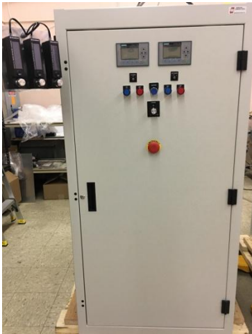
Fig.4. Front door of the APT-100-2 DC module with standard control and 3-gas supply systems
