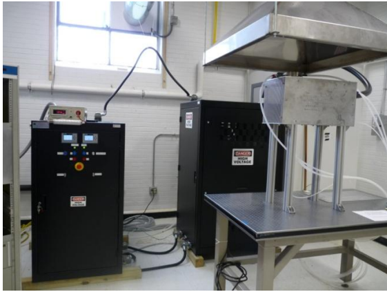
Fig.2. General view of the 100 kW ICP/RF plasma system for material tests.
