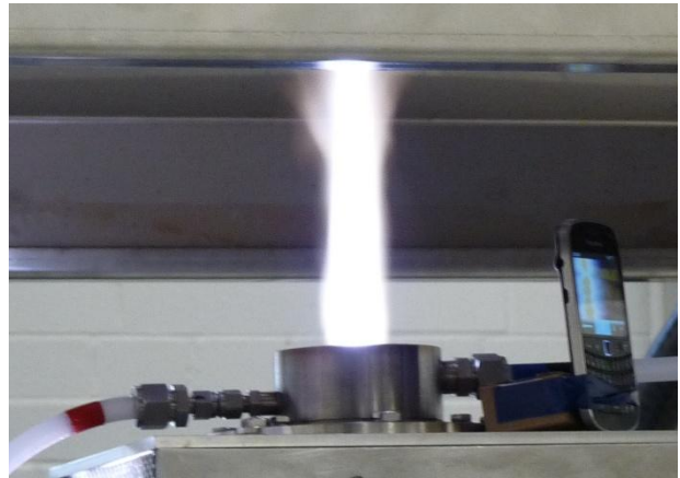
Fig.3. 30 mm OD plasma plume. Gas – air.
