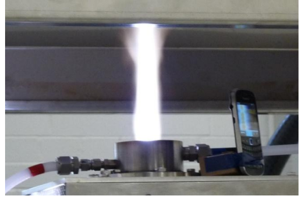
Fig.3. 30 mm OD plasma plume. Gas – air
