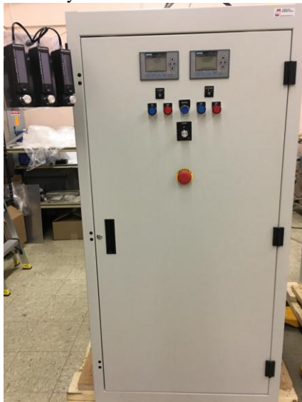
Fig.4. General view of the APT-100-3 DC module with standard control and 3-gas supply systems
