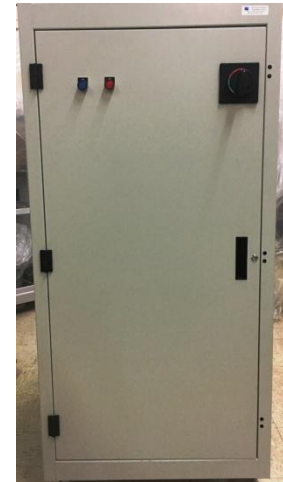
Fig.6. Rear door of the APT-100-5 DC module with remote main power On/Off function
